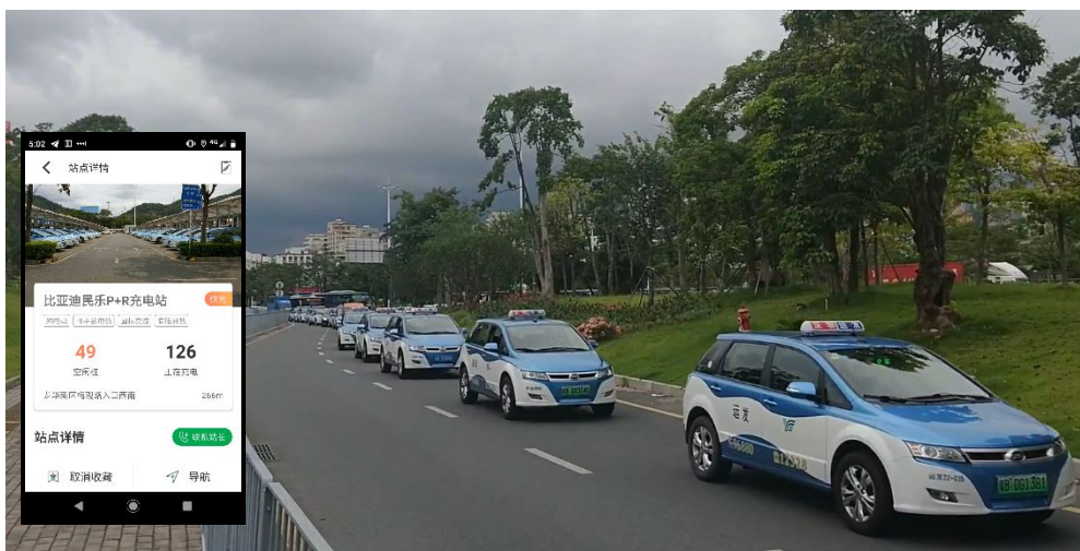
Figure 2. Taxis waiting to charge at Minle station in Shenzhen on July 30, 2019. As shown in the inset, at the same time there were over 100 taxis waiting to charge, a popular charging app by automaker BYD showed 49 available charging ports, suggesting that vehicle data may be necessary to provide real-time charging availability. Minle station is the largest charging station in the world, with over 500 fast chargers, 42 and drivers see it as more reliable than other smaller stations, leading to disparities in usage rates and long queuing times.
