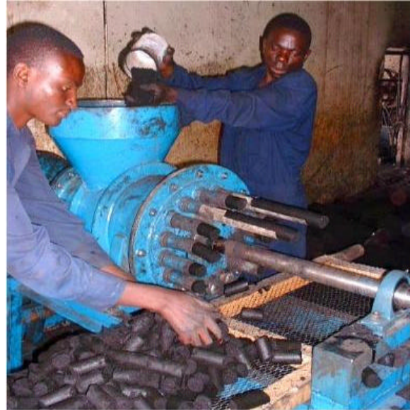
An extruder in operation at Chardust's plant
