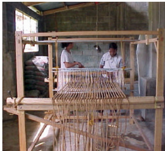
Figure 2: Manufacture of geotextiles from coconut husk fiber
