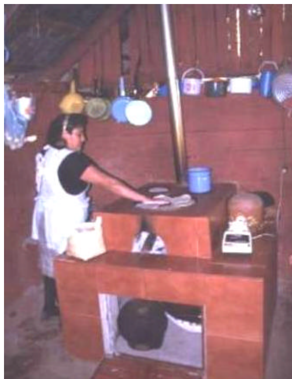
Figure 1. Efficient Lorena-type cookstove shown during tortilla-making. Users' adaptations are almost the rule, in these case a cover has been added to the stove to increase durability and cleanliness.
